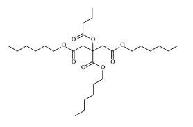
Molecular weight:514.7Melting point:-55°C (pour point)Boiling point:-Vapour pressure:-Solubility in water:< 1g/L at 25°C</td>Log Kow:8.2 (estimated)Purity:>99%Impurities:Volatiles 1.3%, water max 0.15%, heavy metals max. 10 ppm
